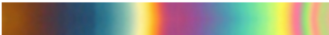
Figure 2.7: Interference colors from a polystyrene film on a silicon wafer which are exactly similar to that of PBLG films [28,61,62]. The film thickness changes from left to right (not on a linear scale): 20 nm (light brown), 70 nm (dark brown), 100 nm (dark blue), 140 nm (light blue) 200 nm (yellow), 250–280 nm (purple), 290 nm (blue), 310 nm (turquoise), 330 nm (green), 350 nm (yellow), 400 nm (light purple), 420 nm (green), 460 nm (yellow), 520 nm (pink) . . . alternating light green and pink up to approximately 1.5 \mu\text{m} until it changes to a transparent gray. Figure adapted from [63].
