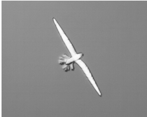
Figure 3.10: An optical micrograph showing a grown PBLG liquid crystal. The experiment was like that of Fig. 3.6. Continuous adding methanol into the thin film solution led to a continuous but slow decrease of \varphi_e which allowed supersaturation ratio S to be bigger than 1. If S > 1 for a long time the object continuously grows to a large size with the length of about 207 \mu\text{m} . Size of the micrograph is 330 \times 264 \mu\text{m}^2 .
